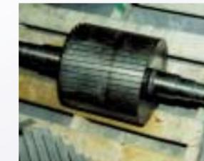
Removing aluminum and cleaning rotors for rewinding.
