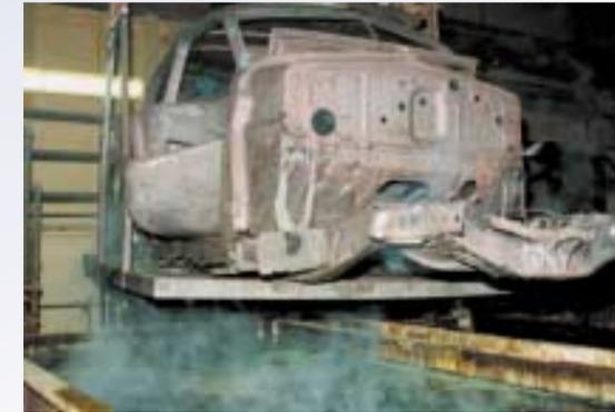
Derusting, stripping and cleaning to base metal car parts and even full size car bodies and frames for old car restoration.
