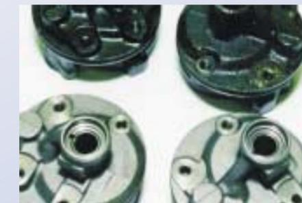
Degreasing and Derusting cast iron parts.
