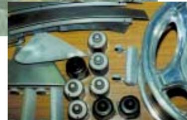
Stripping paint and preparing miscellaneous automotive parts for recoating.
