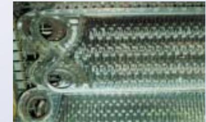
Cleaning stainless steel and titanium heat exchanger plates.
